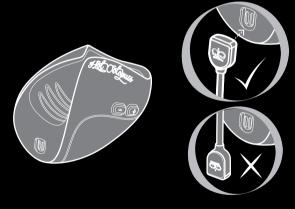
Charge for 4 hours before first use. When cable is attached LED on cable will light RED. When charged LED will turn GREEN. Charger will only work when connected the correct way.
